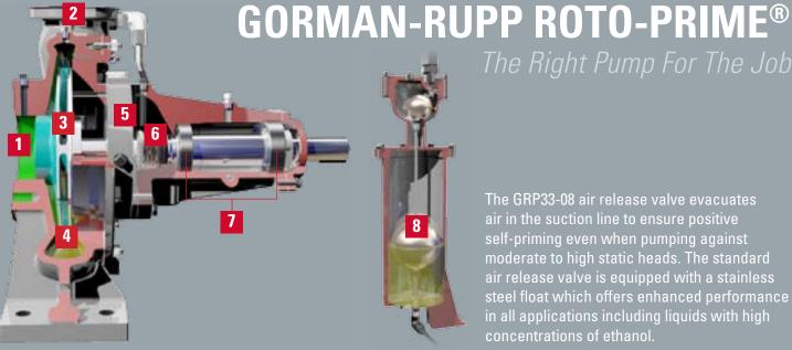
The GRP33-08 air release valve evacuates air in the suction line to ensure positive self-priming even when pumping against moderate to high static heads. The standard air release valve is equipped with a stainless steel float which offers enhanced performance in all applications including liquids with high concentrations of ethanol.
